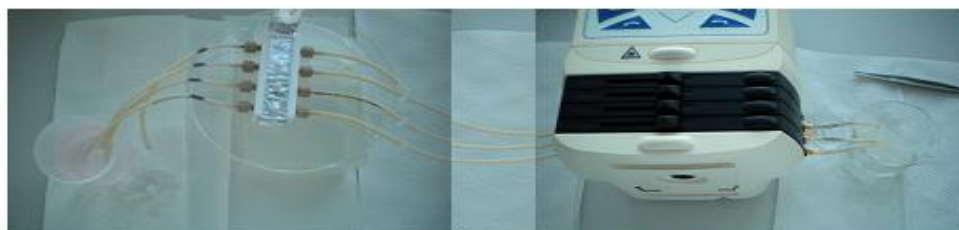
Figure 8: Experimental setup of a 4 channel microfluidic device containing 4 chips: tube ends were dived into the sample or washing buffer, whereas the other end was connected with the Teflon-block. Via peristaltic pump, the fluid was pumped through the channels. The outflow was collected in a waste vessel.
